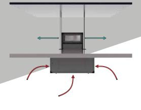
Efficiency HEPA H14 99,995% according to EN1822
