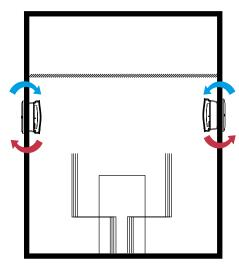
The two heat recovery units they can SUPPLY and EXTRACT air as configured.
