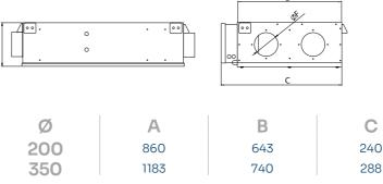
MeasuresAirflow (m³/h)Lp dB(A)InstallationSurface (m²)Applications200/350206/38022,8 - 16,7False ceiling90 - 240Rooms of single<br/>family homes
