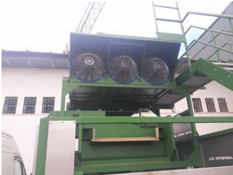
Fan installed in agriculture machine (olives) HB (with poliamide impeller)
