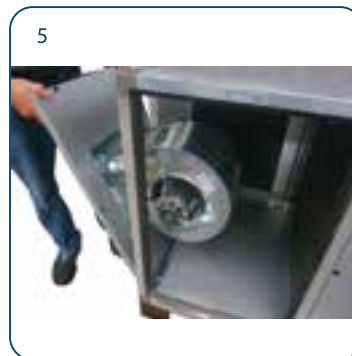
5 Exchange both panels and connect the cables of the fan
