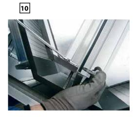
Unscrew the nut and the bolt from the by-pass blade in correspondence of the pin for the external management
